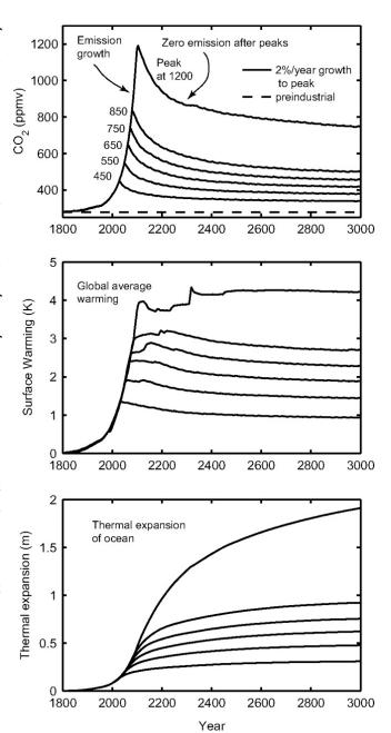
**Figure 2.1.** (Top) Carbon dioxide projections based on the Bern 2.5CC model. CO<sub>2</sub> emissions ramp at a rate of 2%/year to peak CO<sub>2</sub> values listed in the figure. After the peak, emissions are reduced to zero. (Middle) Globally averaged surface warming for the different peak values. (Bottom) Sea level rise due to thermal expansion only. Source. Solomon et al. 2009. Copyright (2009) National Academy of Sciences, U.S.A.
