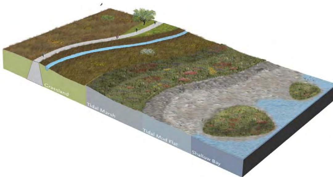
Figure ES-4. Conceptual cross-section of a “horizontal levee”, with an upland ecotone slope bayward of a flood risk management levee and landward of a tidal marsh.
