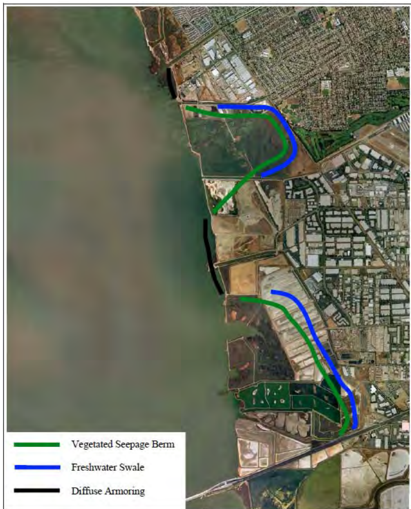
Figure 26. Design elements for a flood protection levee with upland-wetland ecotone.
