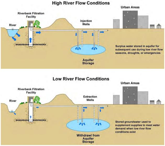
Figure G-9. SCWA Groundwater Banking for High (top) and Low (bottom) River Conditions. Source: Jasperse, 2012.
