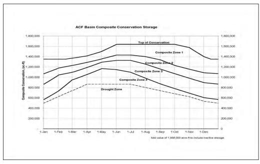
Figure C-6. RIOP Water Storage Zone Levels in the ACF. Credit: USACE Water Management Section, 2014. Source: Crane, 2012.
