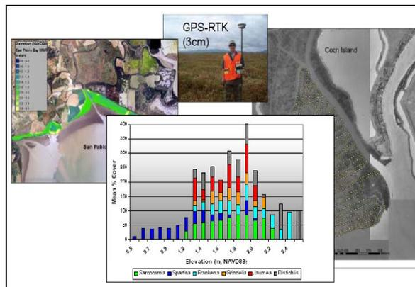
**Figure 3. Elevation and vegetation coverage created from RTK GPS surveys**
